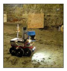
Fig. 3. The Kurt3D robot scanning underground.
